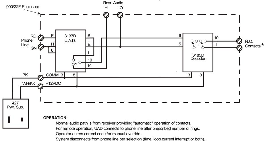
NOTE\* Only one set of Normally Open contacts are shown connected. Additional NO and NC contacts are available on the 3185D card.
